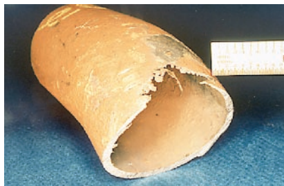
2. Flow-accelerated corrosion can occur in almost all HRSG piping that contains water and water/steam mixtures
