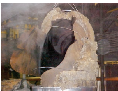
6. Catastrophic failure of feedwater pipe was caused by FAC
