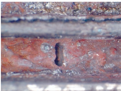
4. Corrosion fatigue is most common in and around economizers, though it also is possible in evaporator sections
