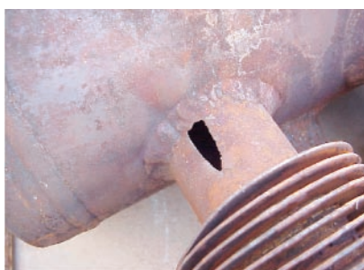
5. FAC in LP evaporator exhibits characteristic teardrop shape
