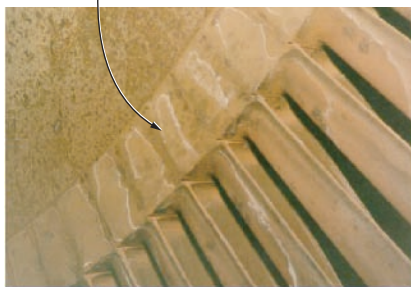
8. Least soluble salts collect in hottest regions of the turbine. Here solute diffuses out of crevice and crystals form on open surfaces
