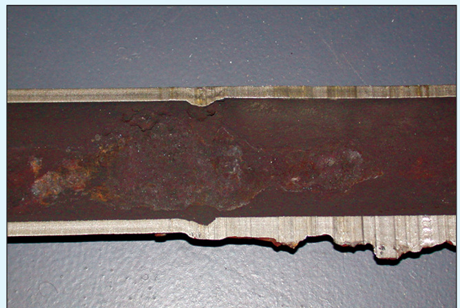
Figure 4: Caustic gouging at a weld.
