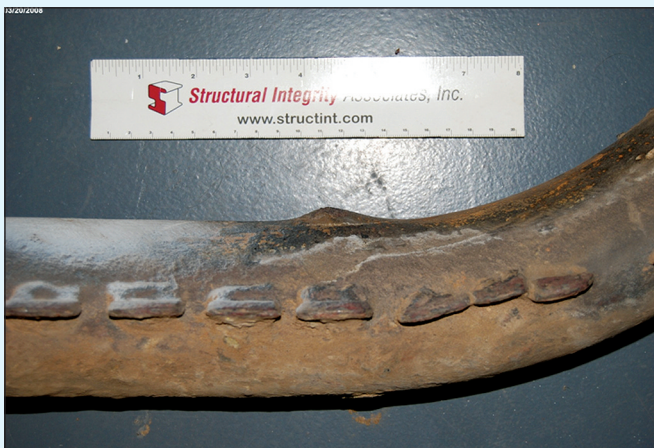
Figure 1: Caustic gouging failure.
