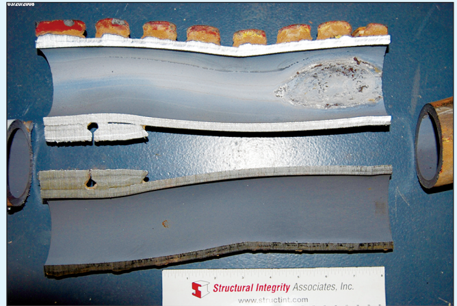
Figure 2: Internal appearance of gouge.
