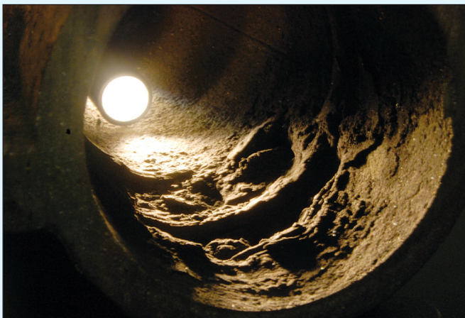
Figure 5: Heavy deposits and caustic gouging.
