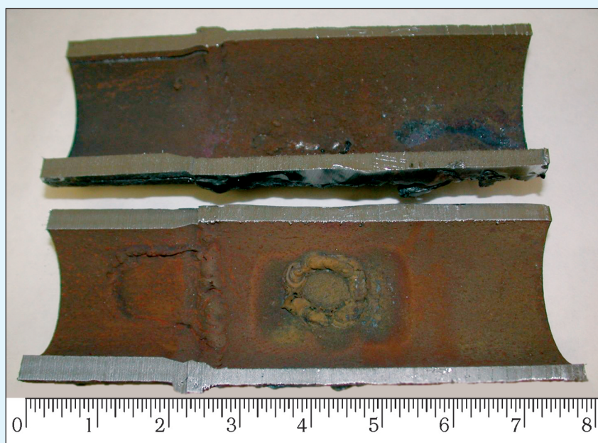
Figure 3: Weld repair showing through to the tube inside becomes a flow disruption.
