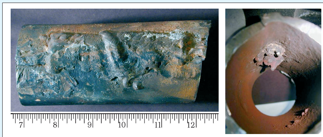
Figure 1: Tube inner surface showing heavy local deposits from penetration of weld repair to the tube inside.
