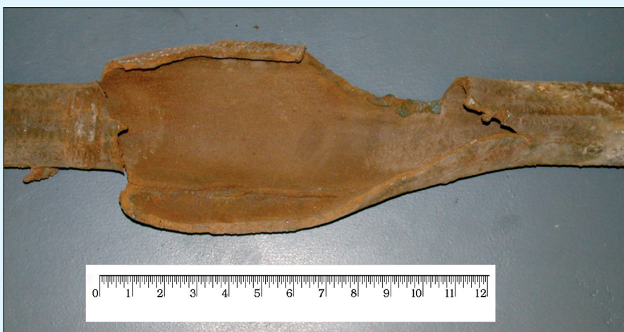
Figure 8: Large hydrogen damage failure.
